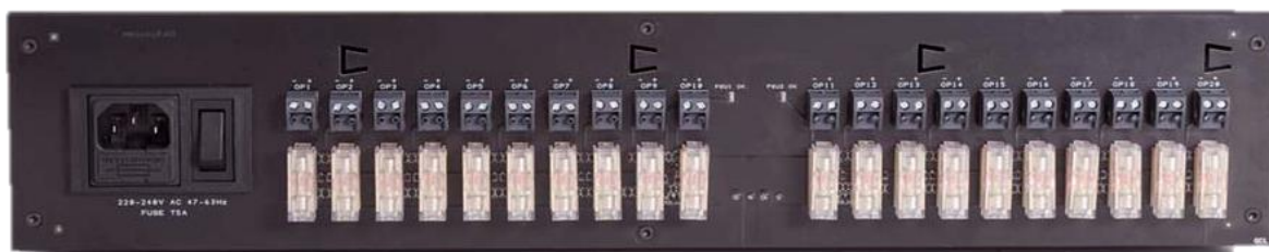
Rear View showing mains input socket, fuses and individual output status LEDs
