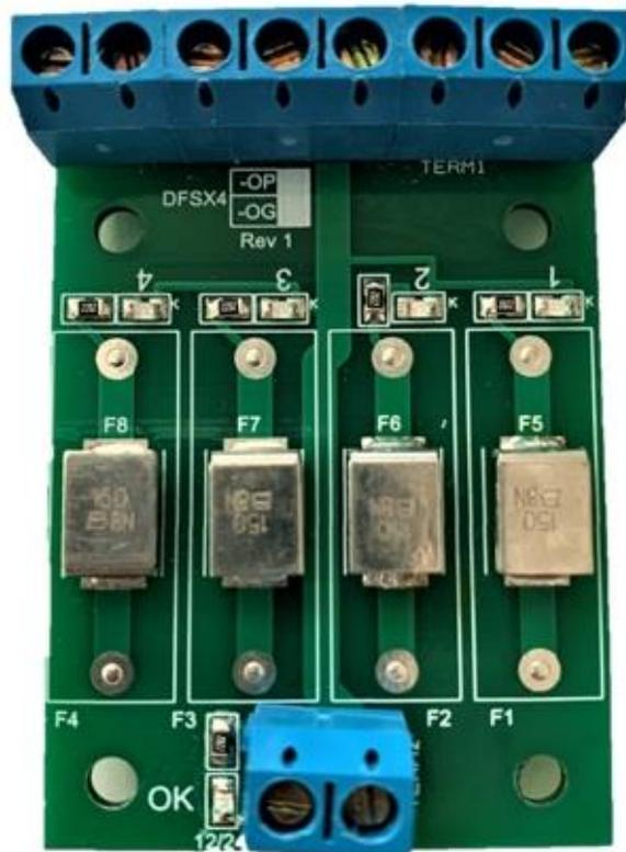
DFX4-OP 4-way, self-resetting, electronically-fused output splitter
