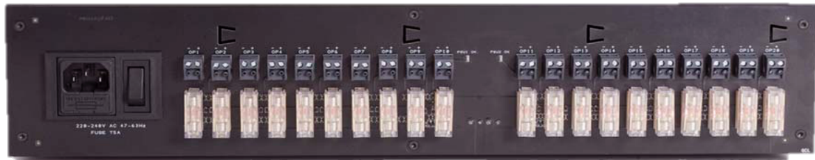
Rear View showing mains input socket, fuses and individual output status LEDs
