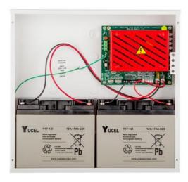
Larger systems require more power, D2433-17 (3A) & D2435 (5A) units), have ample space for 2 x 12VDC 17Ah batteries
