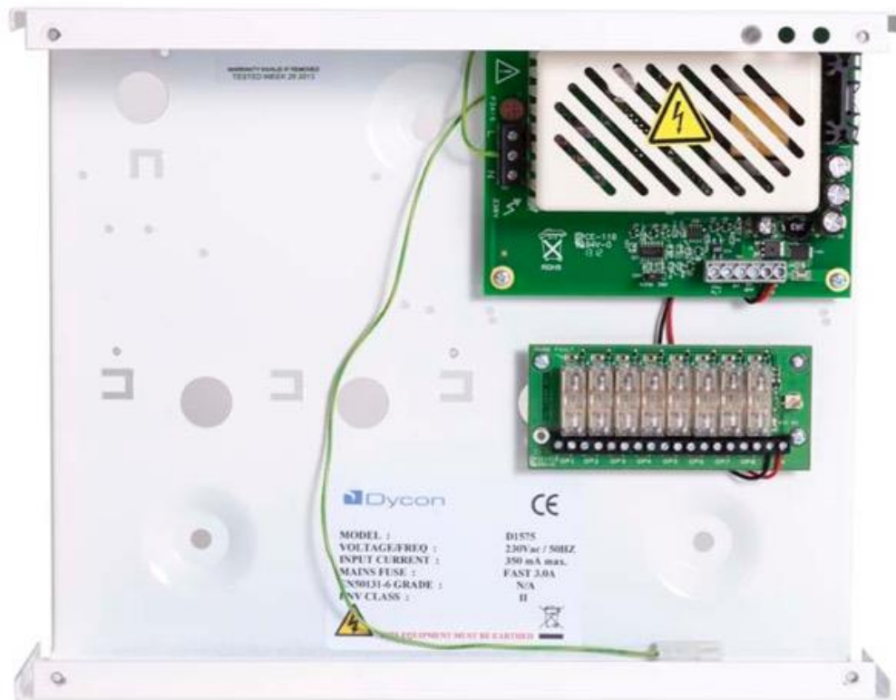
Illustration shows D1575 with an optional D15X8 8-channel output splitter
