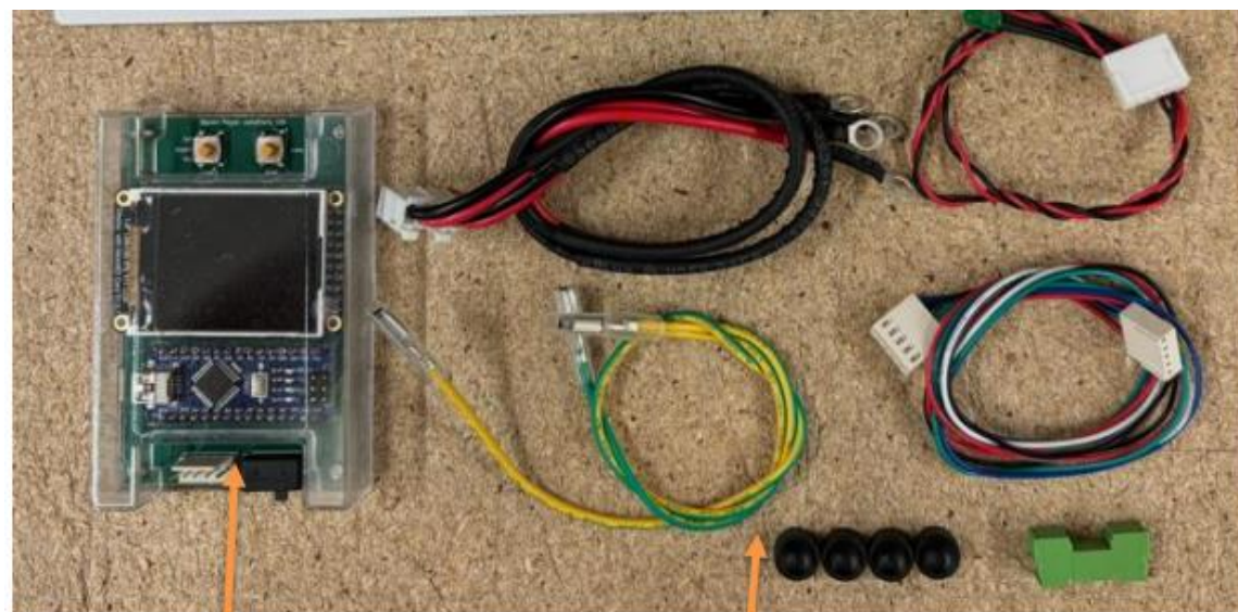
PSUMON-01 Real-Time PSU monitor with colour display
