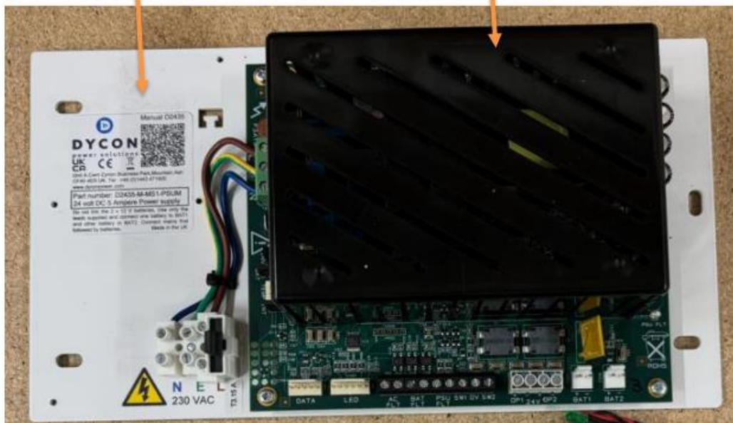
2mm steel plate with PSU and 230VAC mains connector, ready-assembled and wired
