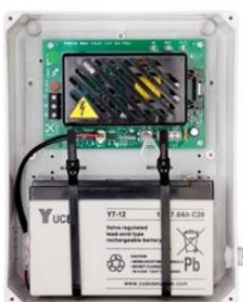
Stage 1 - side & lid removed for basic installation & shows the optional Quick fit' mains option in operation.
