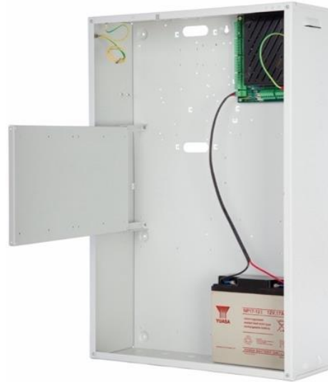
A G-box with a Dycon D1460 10A PSU and a 17Ah VRLA battery, showing the hinged module platform and the ample space for extra peripherals, cables & more batteries.
